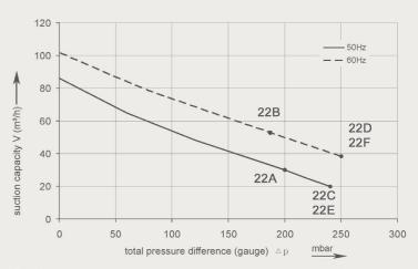
Curves are valid for dry air, with a temperature of 15°C at the inlet and a pressure of 1013 m bar(a) at the inlet or outlet connection (for over- or under-pressure application respectively). The tolerance on capacity is +/- 10%. No rights can be derived from the sketches, dimensions and contents of this data sheet. The data is for information purposes only. Induvac reserves the right to change or modify the data. No complaints can be made about this.
