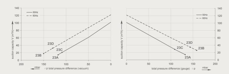
Curves are valid for dry air, with a temperature of 15°C at the inlet and a pressure of 1013 m bar(a) at the inlet or outlet connection (for over- or under-pressure application respectively). The tolerance on capacity is +/- 10%. No rights can be derived from the sketches, dimensions and contents of this data sheet. The data is for information purposes only. Induvac reserves the right to change or modify the data. No complaints can be made about this.
