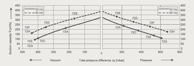
Curves are valid for dry air, with a temperature of 15°C at the inlet and a pressure of 1013 m bar(a) at the inlet or outlet connection (for over- or under-pressure application respectively). The tolerance on capacity is +/- 10%. No rights can be derived from the sketches, dimensions and contents of this data sheet. The data is for information purposes only. Induvac reserves the right to change or modify the data. No complaints can be made about this.
