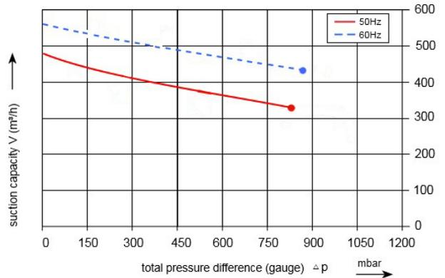
Curves are valid for dry air, with a temperature of 15°C on the inlet side and a pressure of 1013 mbar(a) on the inlet or discharge side connection ( respectively for over and under pressure) The tolerance on capacity is +/- 10%.
